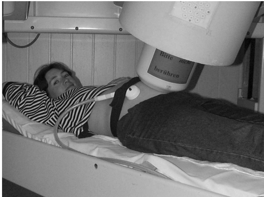
Figure 17.28. A 31-channel SQUID apparatus for fetal cardiography. This investigation is performed in a magnetically shielded room in a hospital. (Courtesy of Dr. Ekkehard Schelußner, Friedrich Schiller University, Jena.)
