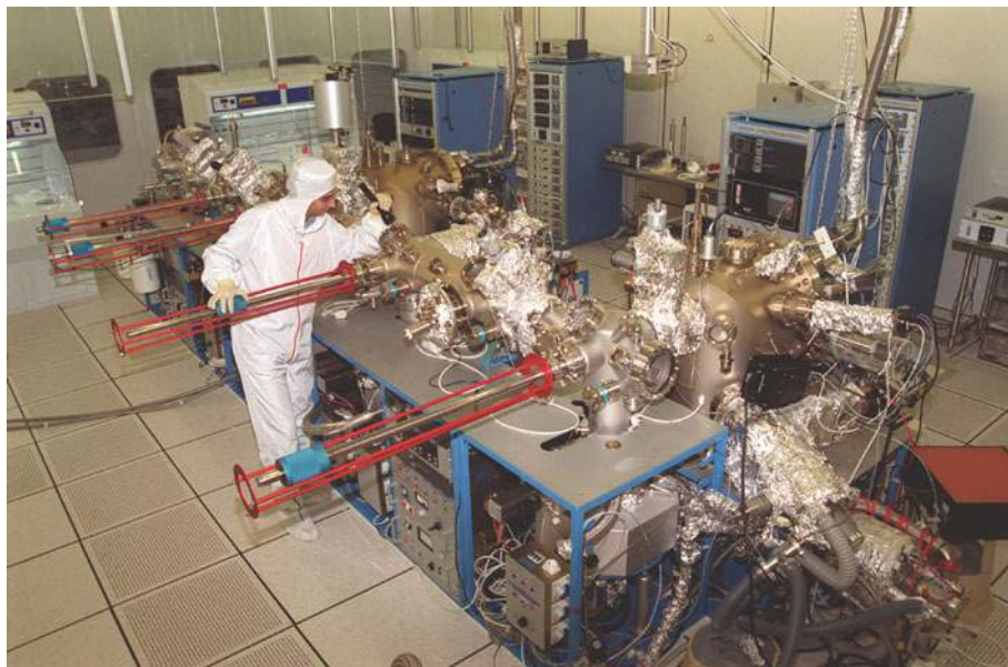
Figure 12.1. A molecular-beam-epitaxy (MBE) growth/analysis system at the Braun Submicron Center at the Weizmann Institute. Inside an ultra-high-vacuum chamber, this method is able to grow epitaxial layers (such as gallium arsenide and aluminum-gallium arsenide) one by one with excellent control over materials and purity. Such layers (produced using MBE, or often less exacting methods) form the basis of many semiconductor devices.
