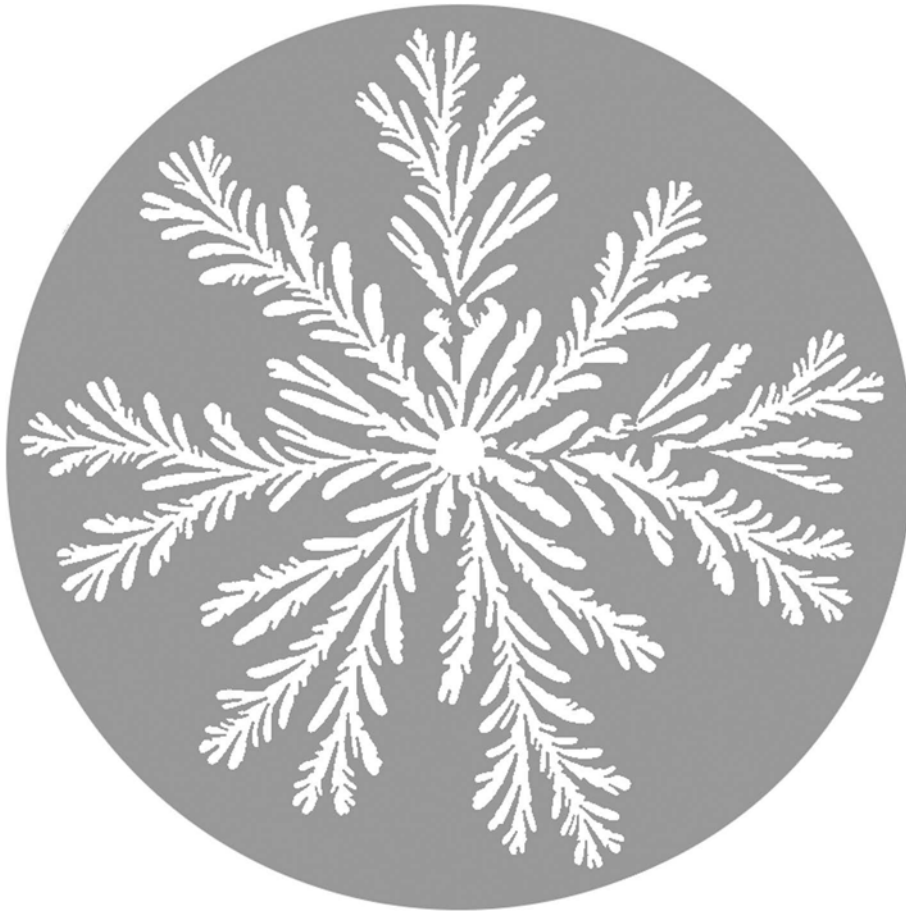
Figure 14.12. A pattern formed by pumping air into an oil layer contained between two 300-mm-diameter glass plates spaced only 0.13 mm apart. (Courtesy of M. G. Moore, E. Sharon, and H. L. Swinney, University of Texas at Austin.)
