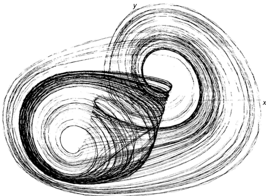
Figure 13.5. The reconstructed attractor of the behavior shown in Figure 13.4. The coordinates (x, y, z) are (V(t), V(t - \tau), V(t - 2\tau)) , where the time lag is 4.5 ms. Knowing the form of the attractor, prediction becomes possible within the limits set by the largest Lyapunov exponent.
