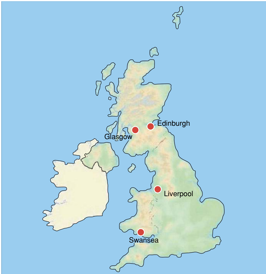
Figure 15.3. The UK QCDGrid system has data nodes at four sites to provide multi-terabyte storage for quantum-chromodynamics calculations of particle properties. To safeguard data, no one node is independent of the others. The data are replicated across the system so that if a node were to fail the data could be recovered. (Courtesy of Tony Doyle, University of Glasgow.)
